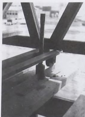
fig. 224: Detail of the simple displacement devices. Metal wheels and rails are used for horizontal movement; metal screws, for vertical displacement.
